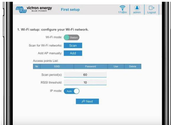
If the Station WiFi mode is enabled, a WiFi strength indicator between the EV Charging Station and the main WiFi is placed at the top of the web page.
